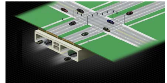
3 Cut and cover tunnel below rebuilt Huron Church Road/Highway 3 Corridor.
