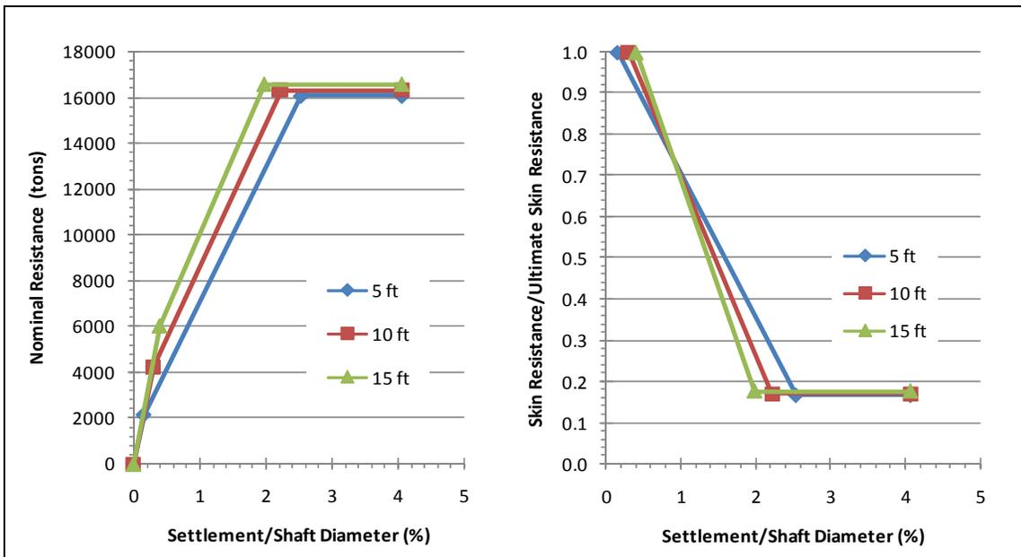
**Figure No. 10-6: Drilled Pier Results Summary for a Diameter of 2.5 m (8.2 ft).**
