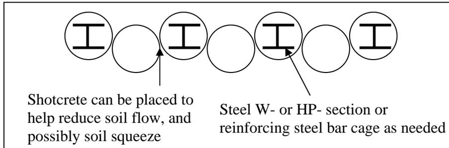
**Figure No. 10-8: Schematic Plan View of a Typical Tangent Pile Wall.**
