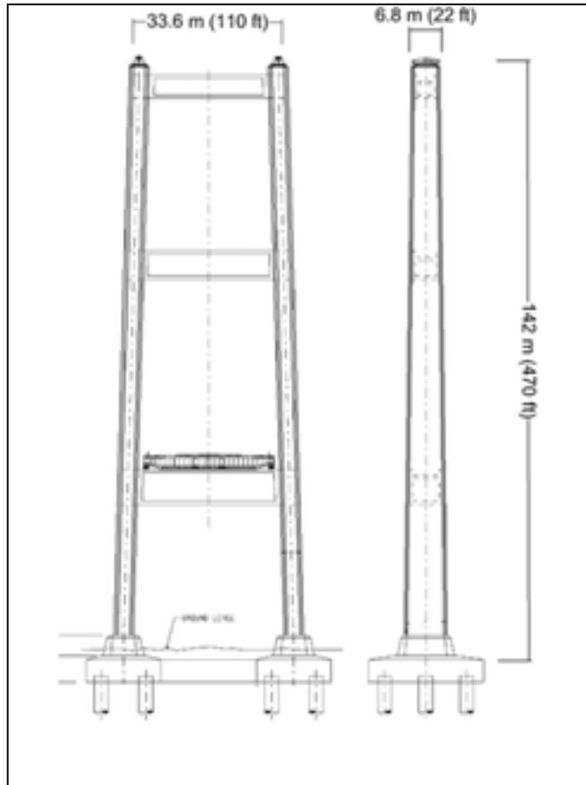
**Figure No. 4-3: Typical Suspension Bridge Tower Configuration**
