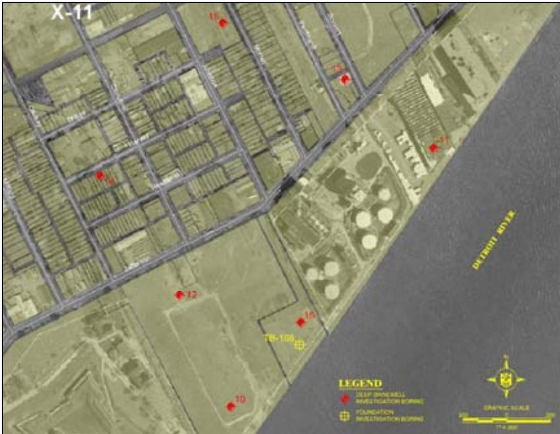
**Figure No. 5-2: Test Boring Location Plan for Crossing X-11.**
