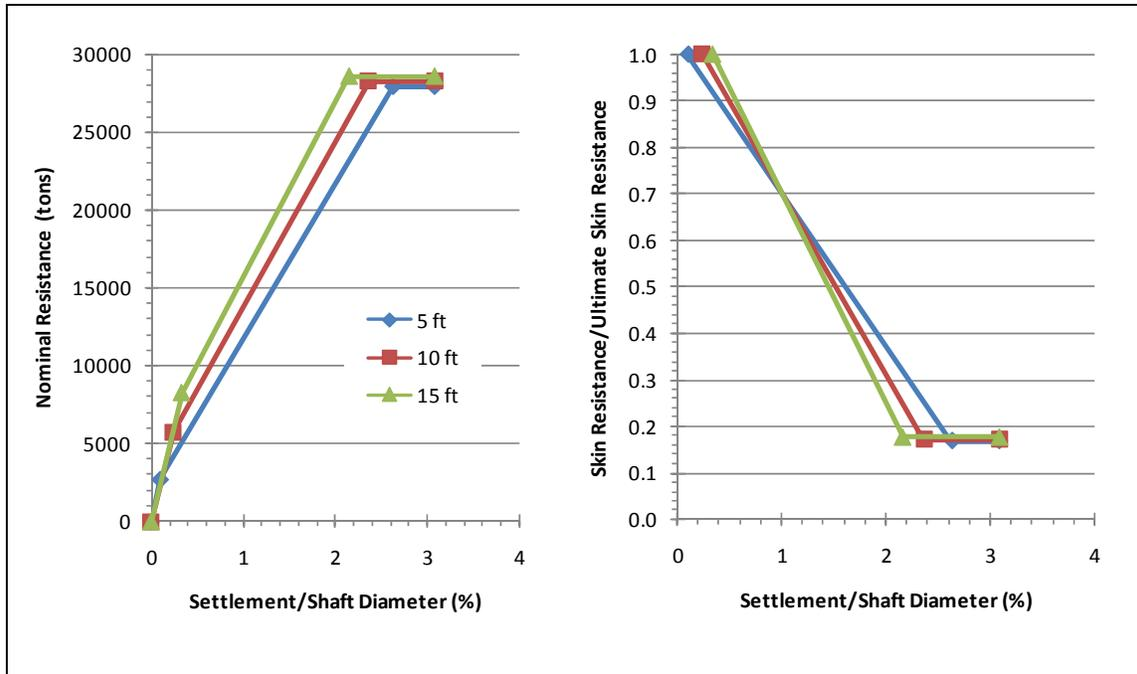
**Figure No. 10-7: Drilled Pier Results Summary for a Diameter of 3.3 m (10.8 ft).**
