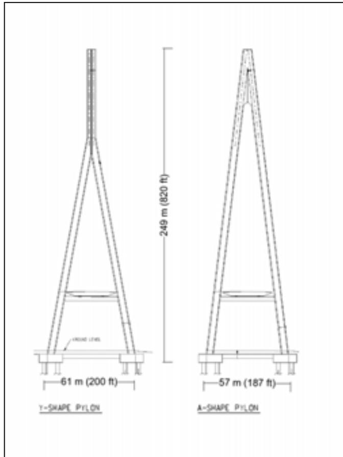
**Figure No. 4-5: Typical Cable-Stayed Bridge Pylon**
