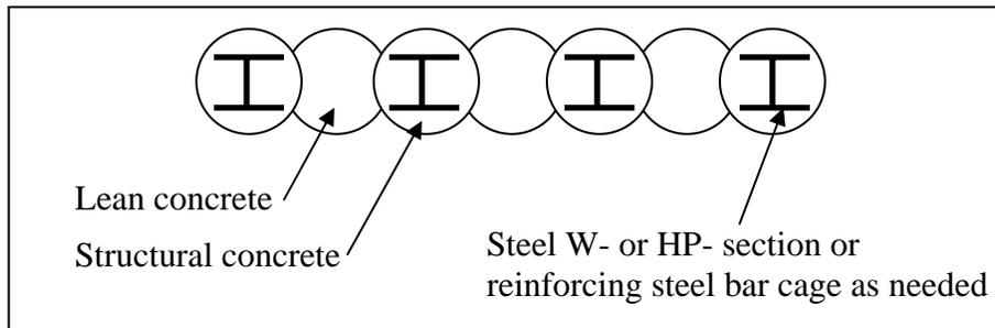
**Figure No. 10-9: Schematic Plan View of a Typical Secant Pile Wall.**
