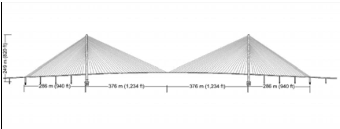
**Figure No. 4-2: Typical Cable-Stayed Bridge Structure**
