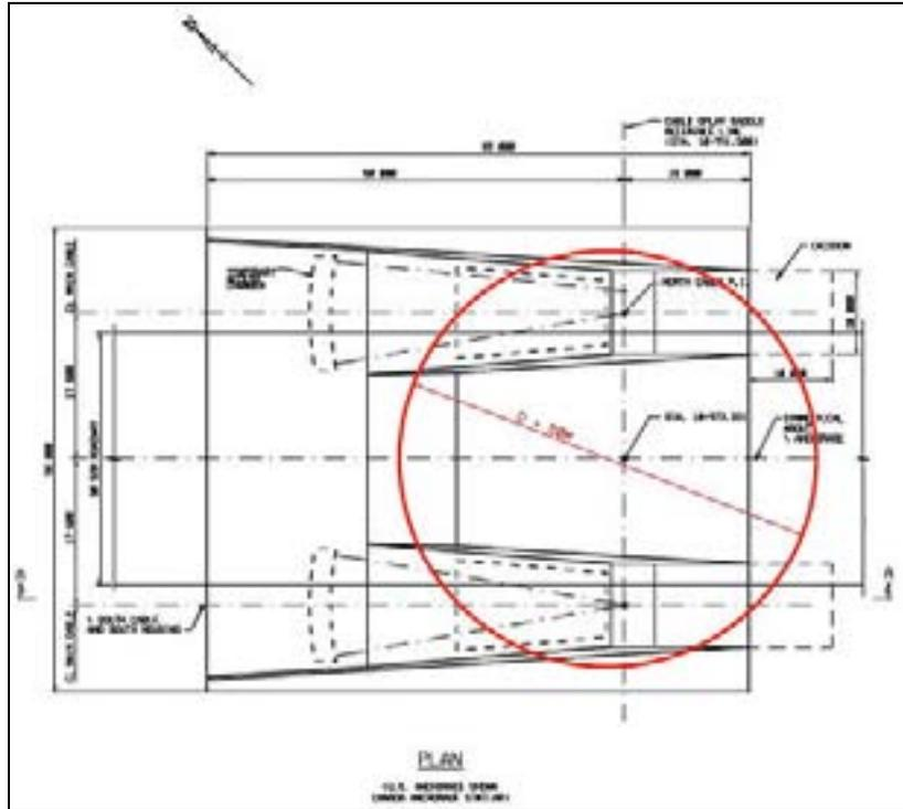
**Figure No. 10-2: Schematic of Option II – Single Circular Caisson.**
