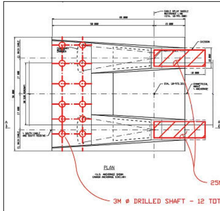
**Figure No. 10-4: Schematic of Option IV – Drilled Shafts and Two Rectangular Caissons.**
