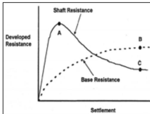
**Figure No. 10-5: Load-Settlement Behavior under Compression Loading (FHWA-IF-99-025).**
