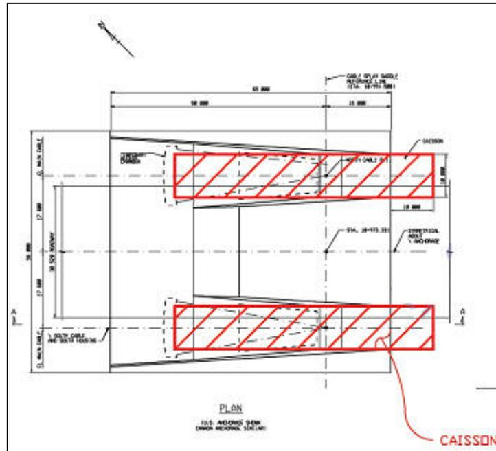
**Figure No. 10-1: Schematic of Option I – Two Rectangular Caissons.**
