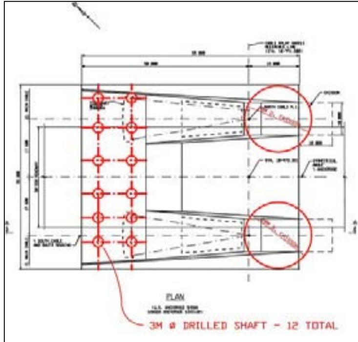
**Figure No. 10-3: Schematic of Option III – Drilled Shafts and Two Circular Caissons.**
