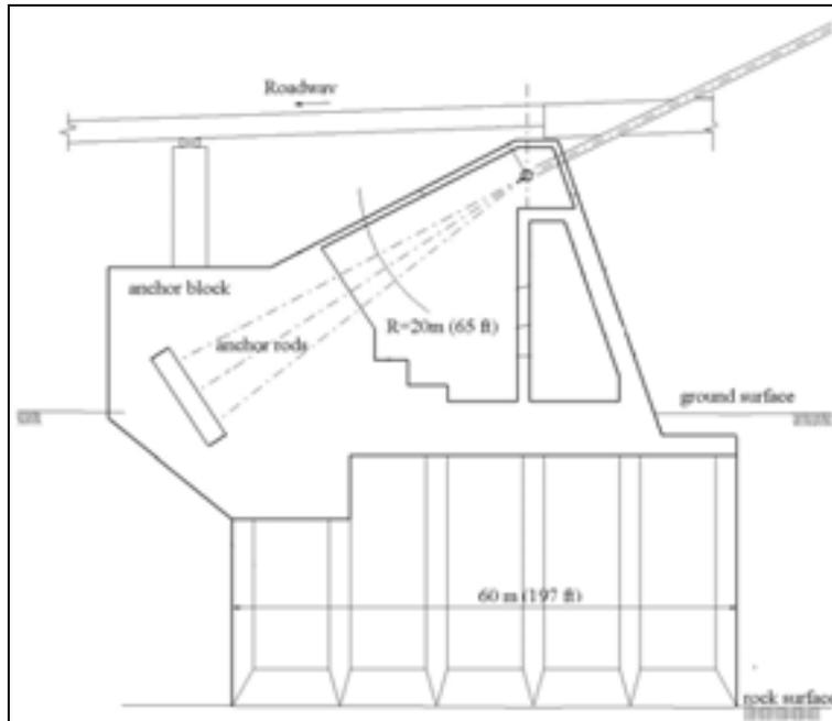
**Figure No. 4-4: Typical Suspension Bridge Anchorage Structure**
