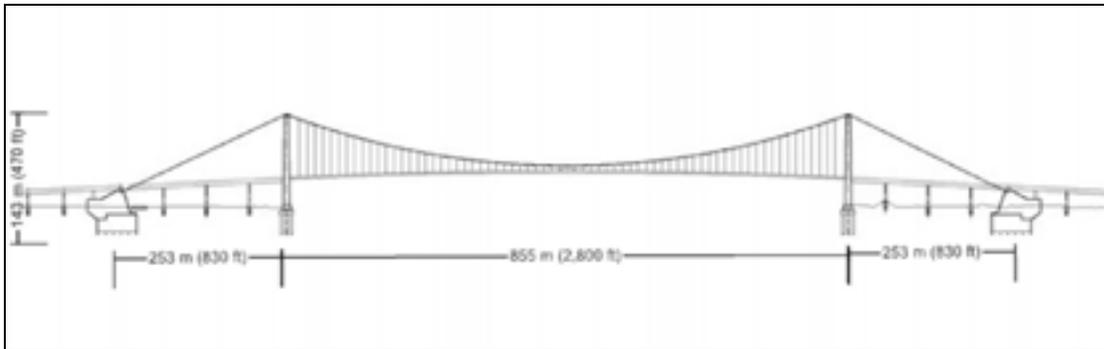
**Figure No. 4-1: Typical Suspension Bridge Structure**
