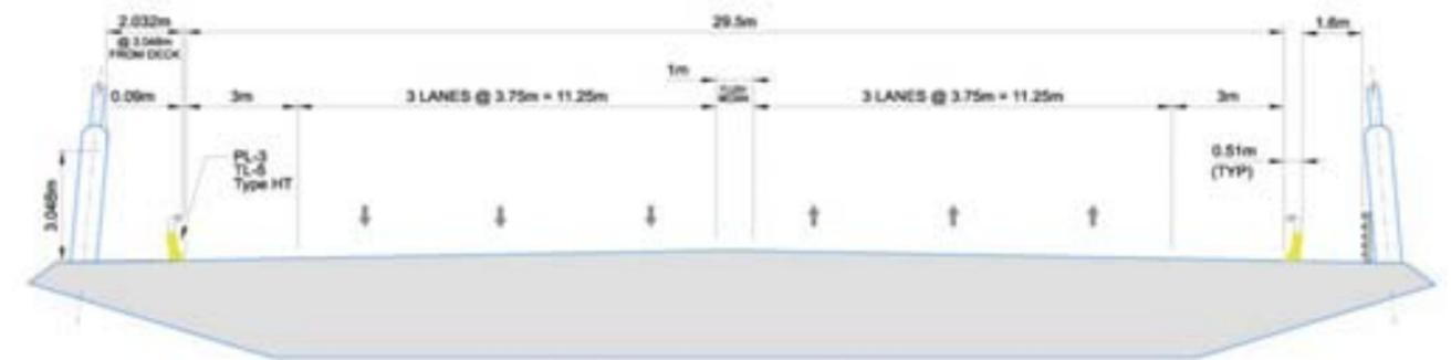
**Figure 8: Proposed Main Bridge Cross Section**
