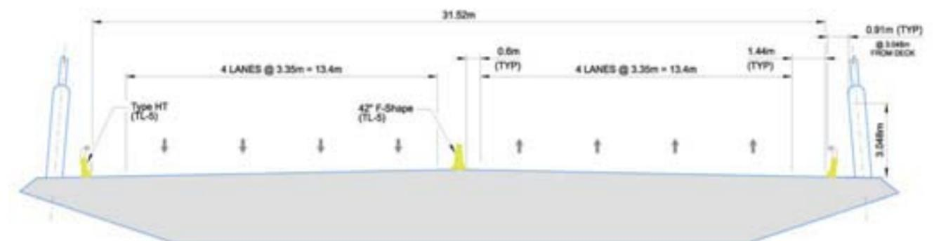
**Figure 9: Future Design Allowance Main Bridge Cross Section**
