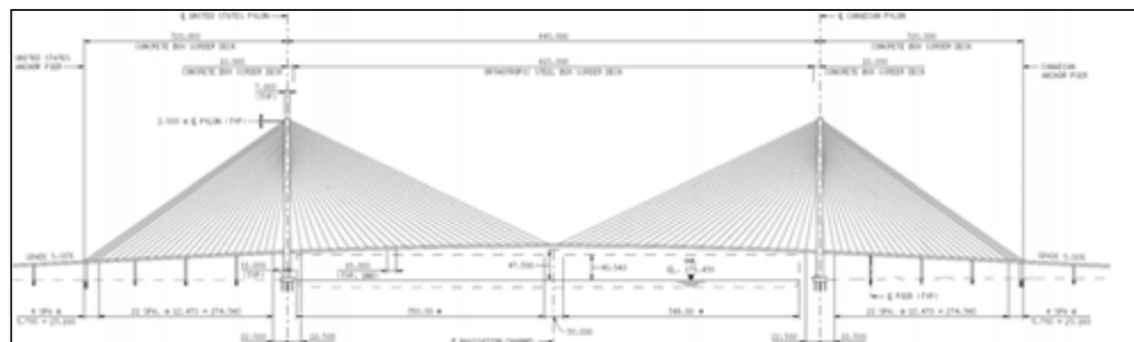
Figure 3: X-10(B) Option 4 Cable-Stay Bridge Elevation
