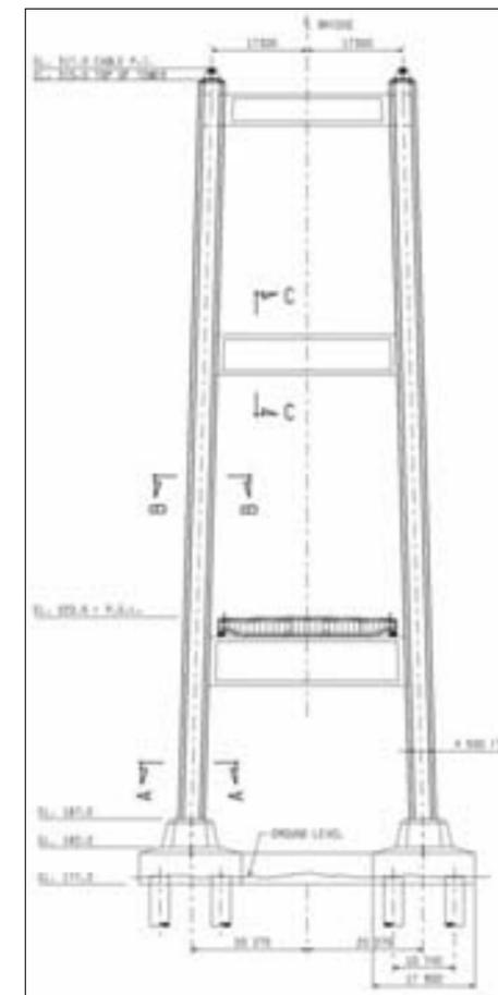
**Figure 10: Suspension Bridge Tower**
