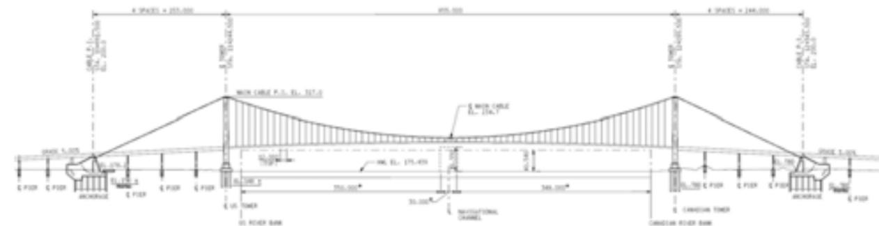
**Figure 2: X-10(B) Option 7 Suspension Bridge Elevation**
