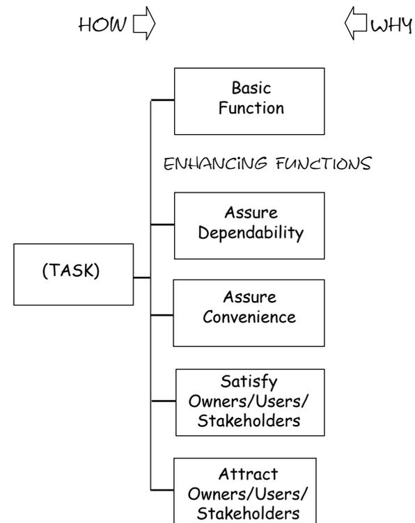
Structure of Function-Logic Diagram
