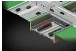
2b Six-lane freeway below grade, parallel to Huron Church/Highway 3:
