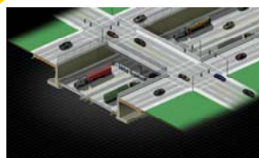
1b One-way service roads either side of 6-lane freeway below grade:
