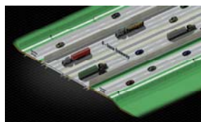
1a One-way service roads on either side of 6-lane freeway at grade:
