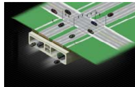
3 Cut and cover tunnel below rebuilt Huron Church Road/Highway 3 Corridor:
