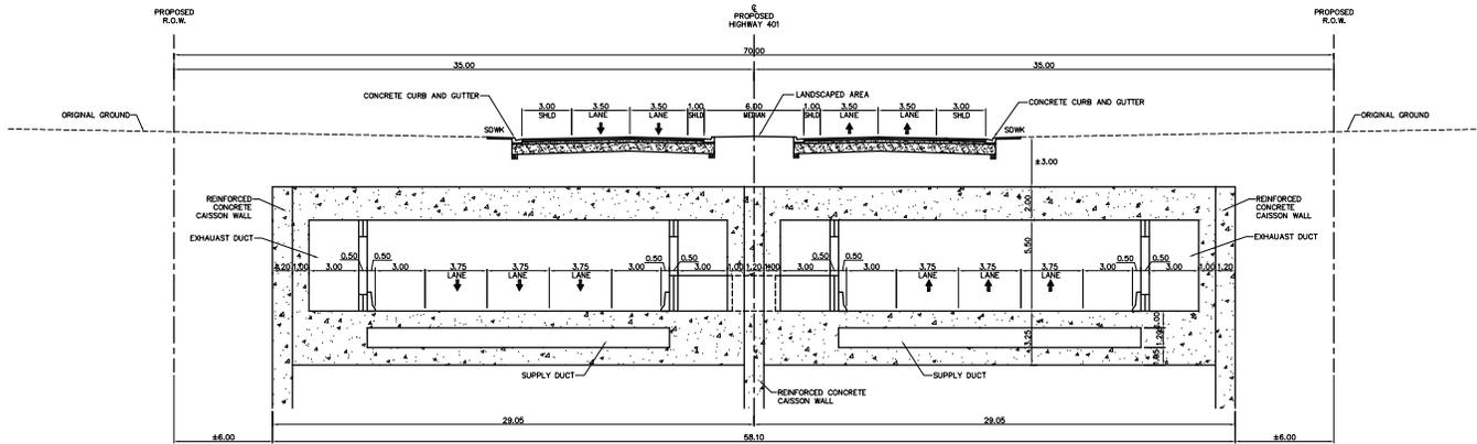
CUT AND COVER TUNNEL SECTION WITH MUNICIPAL DRAIN
