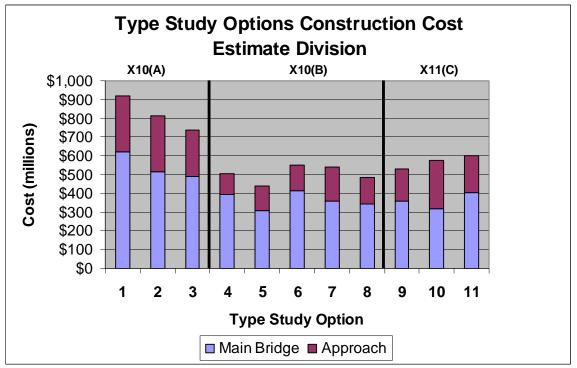
Figure 11. Construction Cost Estimate (Max.) Approach/Main Span Division Graph.
