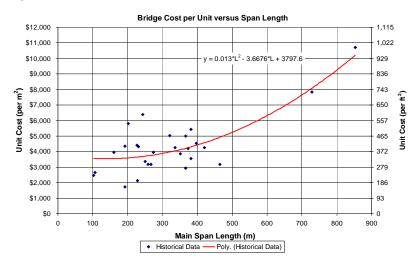
Figure 8. Historical bridge unit costs versus span length.
