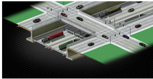
1B One-way service roads either side of 6-lane freeway below-grade.
