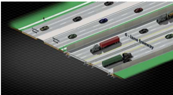
2A Six-lane freeway at grade, along side Huron Church/Highway 3.
