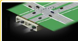
3 Cut and cover tunnel below rebuilt Huron Church Road/Highway 3 Corridor.
