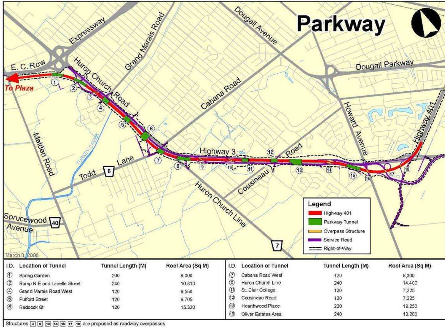
FIGURE 1.2 THE WINDSOR-ESSEX PARKWAY TUNNEL CONFIGURATIONS
