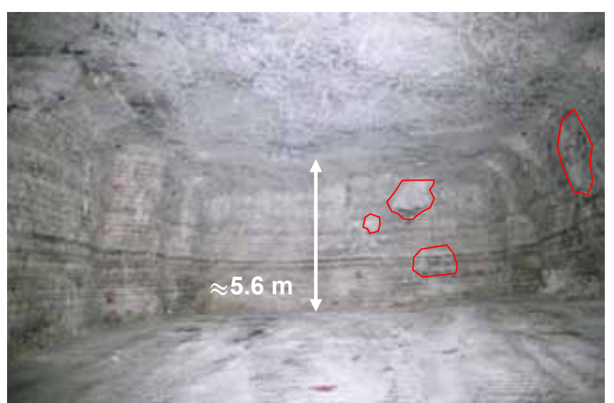
Zones of natural dissolution and recrystallisation of salt outlined in red. Photos taken in Salina Formation F salt.
