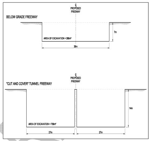
FIGURE 2 - DEPTH AND UNIT AREA FOR EXCAVATION
