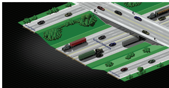
One-way service roads on either side of 6-lane freeway, below-grade. *
