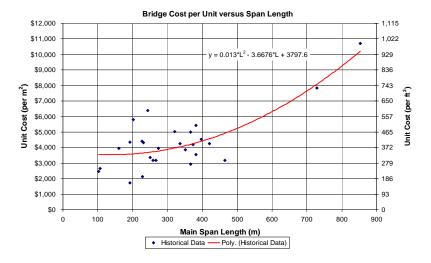
Figure 8. Historical bridge unit costs versus span length.
