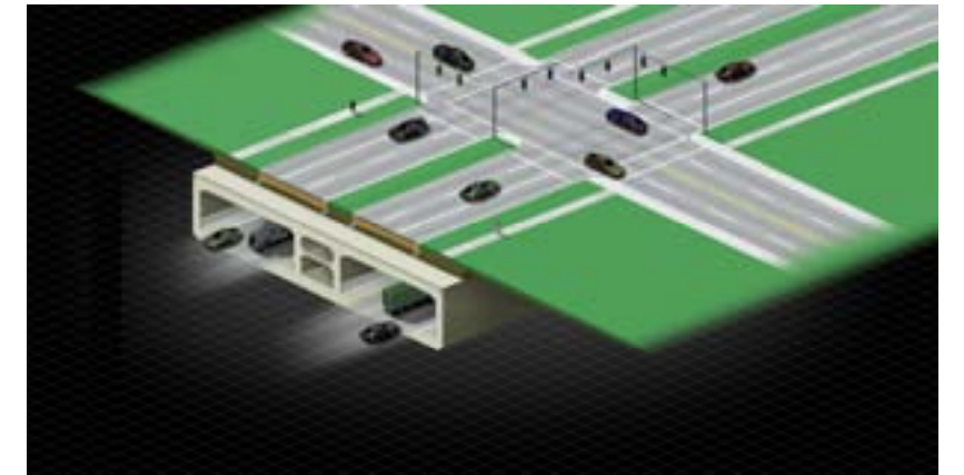
③ Cut and cover tunnel below rebuilt Huron Church Road/Highway 3 Corridor.
