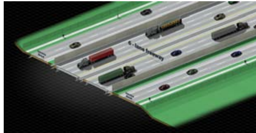
① One-way service roads on either side of 6-lane freeway at grade.
